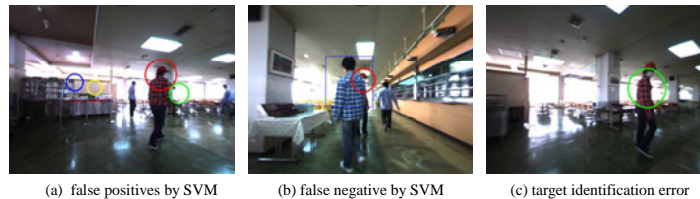
Figure 10. Visual person detection errors.
